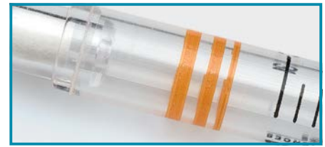
Volume identification by color coding on pipette enables easy volume identification during working.
