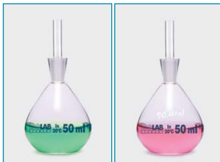
Net volume with 0,001 ml precision is engraved on the body of calibrated density bottles.
