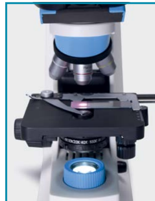
142x138 mm square mechanical stage with 76 mm left-right and 55 mm back-forward movement offers easy use.
