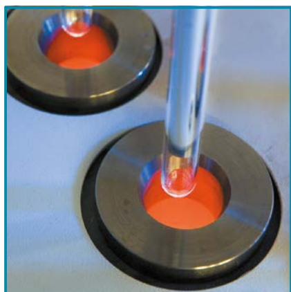
Glass tubings are slowly and gradually heated up to half-melting level. Then they are shrunk around steel rods with precise diameter.
